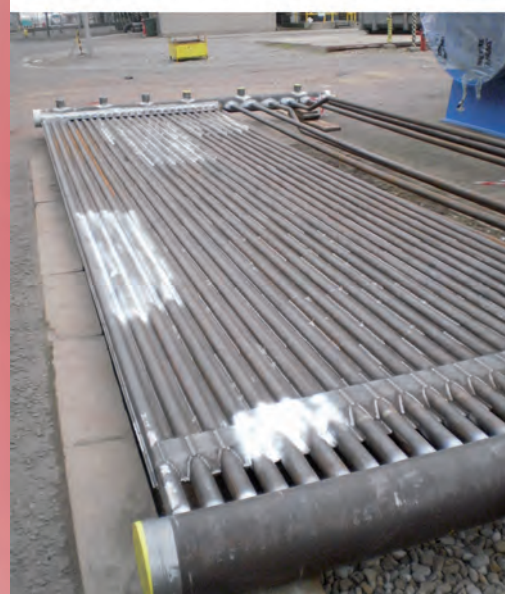
INEOS - Fabricated superheater protection wall header
