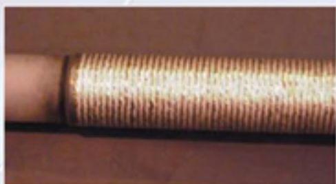
Close up - 2.5mm thick Inconel 625 welded automatically onto 15Mo3 boiler tube.
