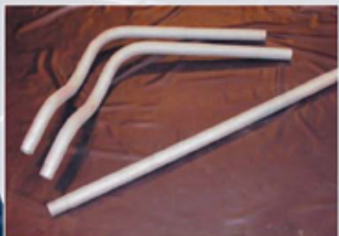
Wall tube - after weld overlay and manipulation.
